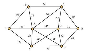
**Problem:** The vertices represent 8 regional data centers which need to be connected with high-speed data lines. Feasibility studies show that the links illustrated above are possible, and the cost in millions of dollars is shown next to the link. Which links should be constructed to enable full communication (with relays allowed) and keep the total cost minimal.
